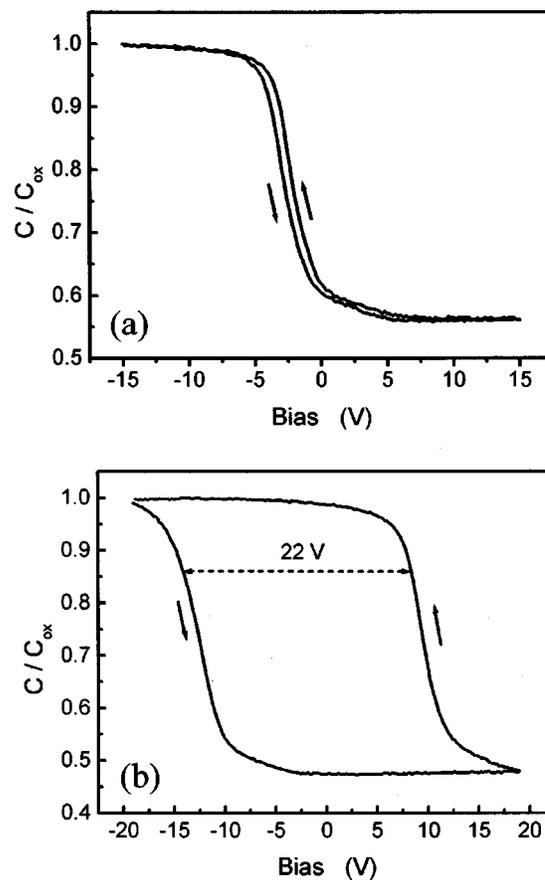
FIG. 2.  $C$ – $V$  characteristics of EBD sample (a) and IBAED sample (b). A dual sweeping mode is employed for  $C$ – $V$  characteristics. Arrows in the figures are sweeping directions, sweeping rate was 2 V/s.
